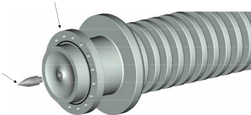
Fig. 5.11: Perspective view of the intended insulator. The cathode is removable.
