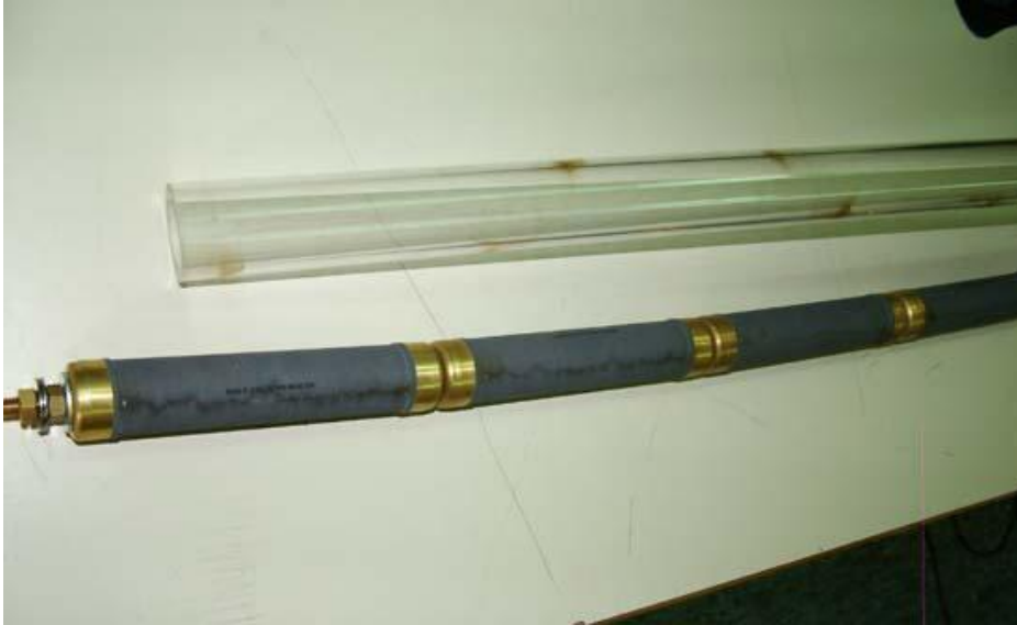
Fig. 7.32: High voltage divider resistors. Distinguished mark of your erpou- discharge surface resistances and signs in acrylic tube.
