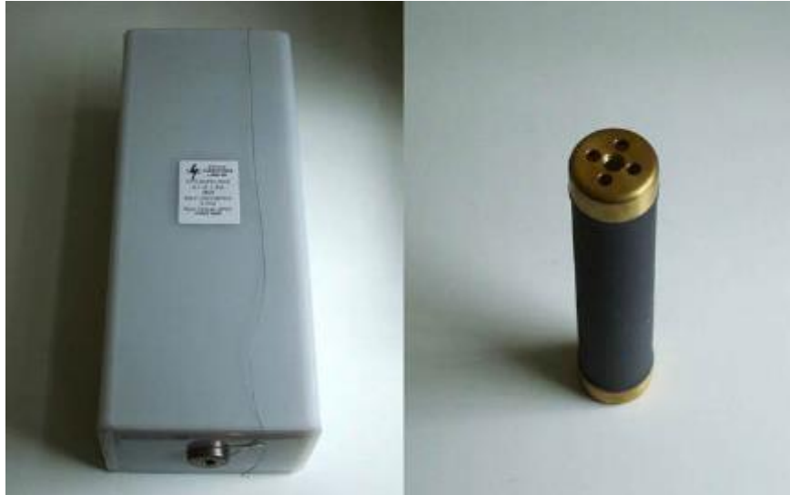
Fig. 7.2: Capacitor discharge impulse 50kV (left) and resistance 70kV, 55W (de- Xia). The resistors 1MO and 10MO have identical dimensions.
