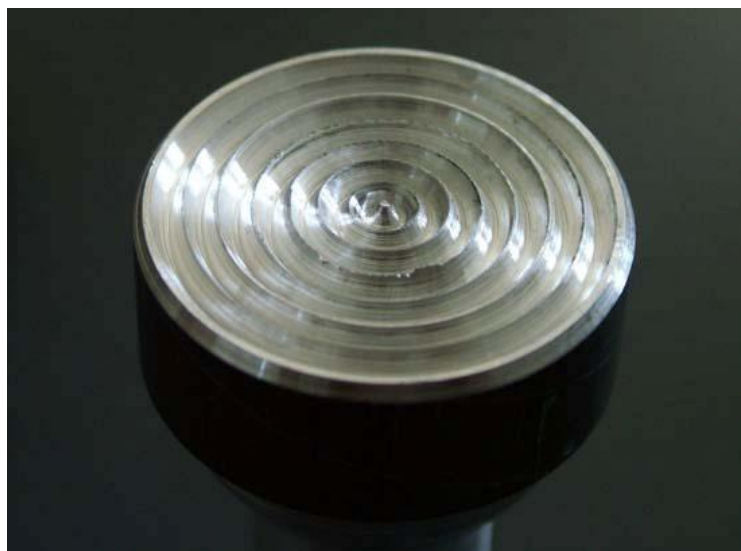
Fig. 6124: Descent grooved, d_{AK} = 14\text{mm} .
