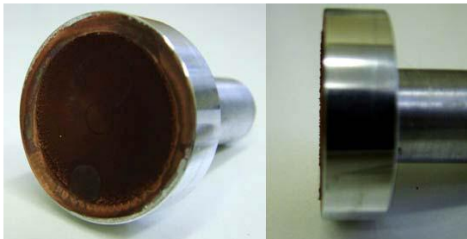
Fig. 7.42: Cylindrical cathode copper accretion.
