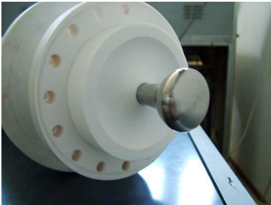
Fig. 6.100: Ductile cathode d_{AK} = 15 \text{ mm} , mounted on the insulator passage.
