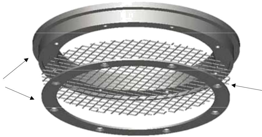
Fig. 5.16: The fixture of metal mesh anode.
