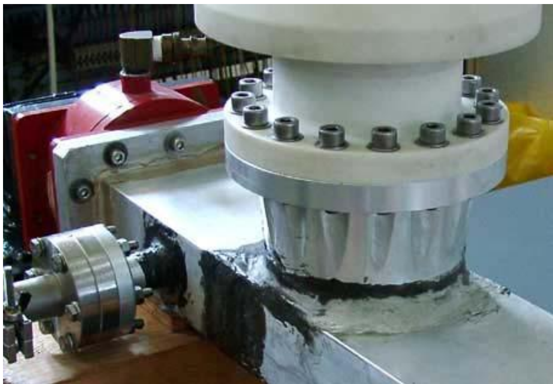
Fig. 5.26: Coating resins in order to reduce leakage in the compounds of the lamp.
