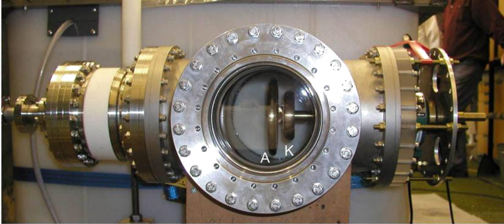
Fig. 4.23: Vircator type Reflex Triode. The pulse is driven to rise. Left is customized vacuum pump (not visible) through a dielectric ceramic liaison bodies, for electrical isolation of the pump from the impulse land [116].
