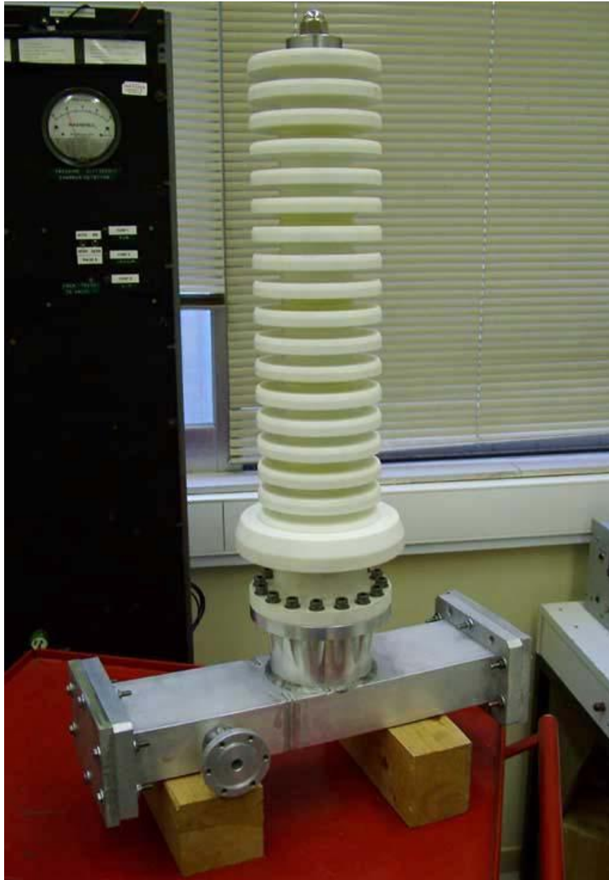
Fig. 5.2: The Vircator, as received from the machine shop.
